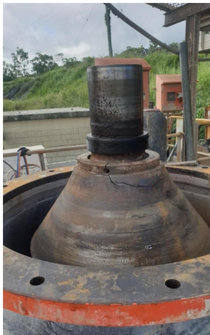
Fig 5&6 Broken Main Shaft of the Secondary Gyratory Crushing Unit
