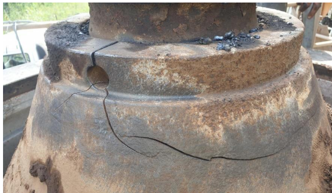
Fig 5&6 Broken Main Shaft of the Secondary Gyratory Crushing Unit
