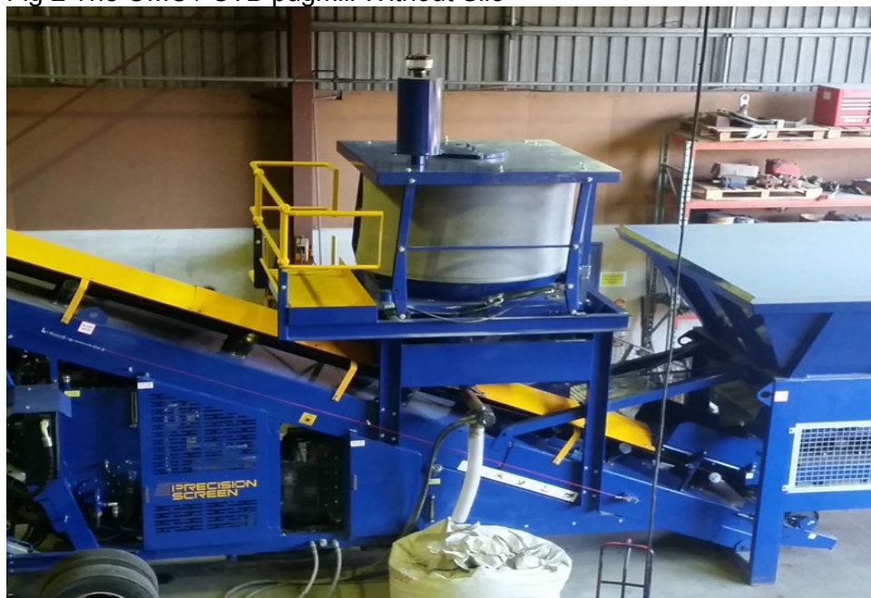
Fig 2 The OMC / CTB pugmill Without Silo
