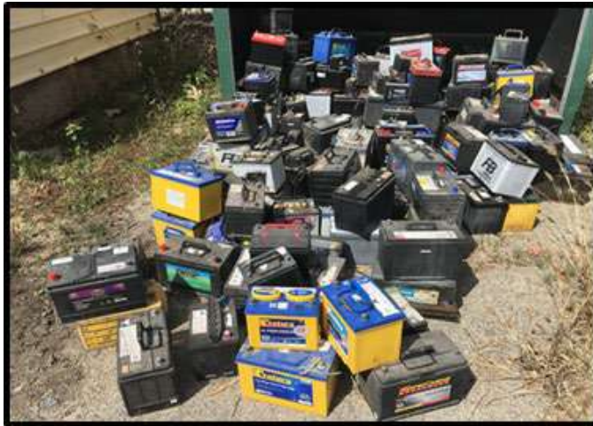
Before: Poor storage practice
