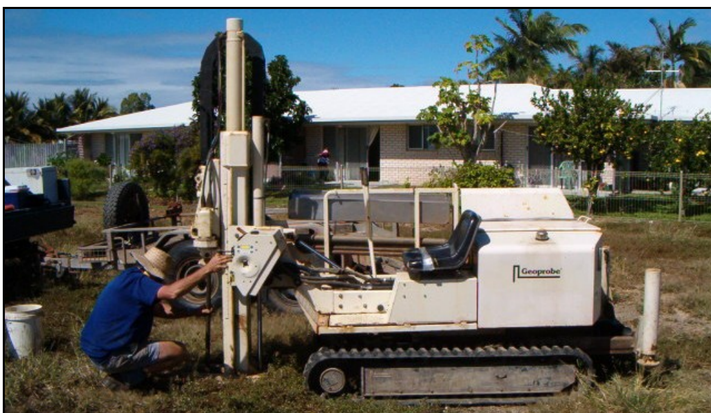
Photograph 4. Geoprobe® used for deep sediment sampling
