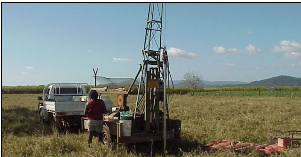
Photograph 3. Trailer mounted vibro-coring soil rig used for sampling wet sediments
