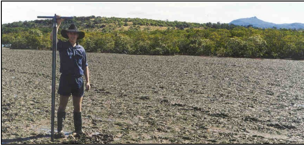
Photograph 2. Gouge auger, 1.8 m long, used for hand sampling in mangrove forests and salt pans
