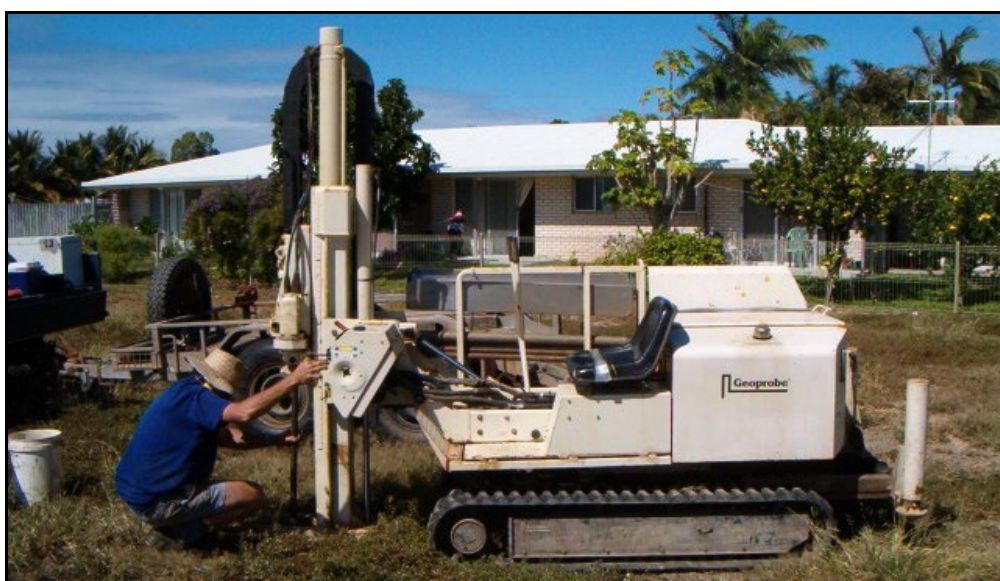
Photograph 4. Geoprobe® used for sampling the very gravelly soils
