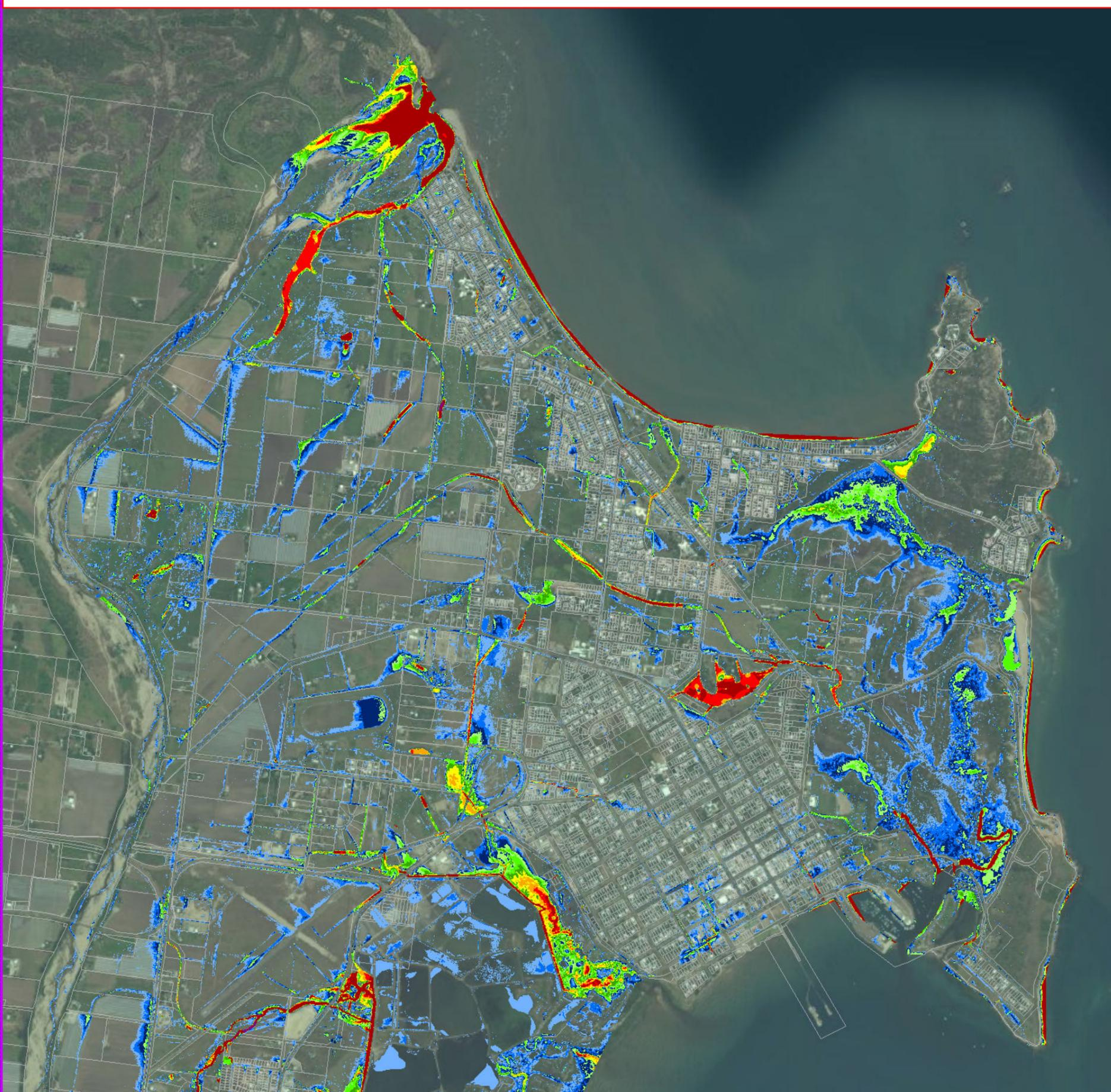
All flood maps are based on Bowen Local Catchment Flooding only. The impacts from Storm Surge and Riverine Flooding should be considered separately.
