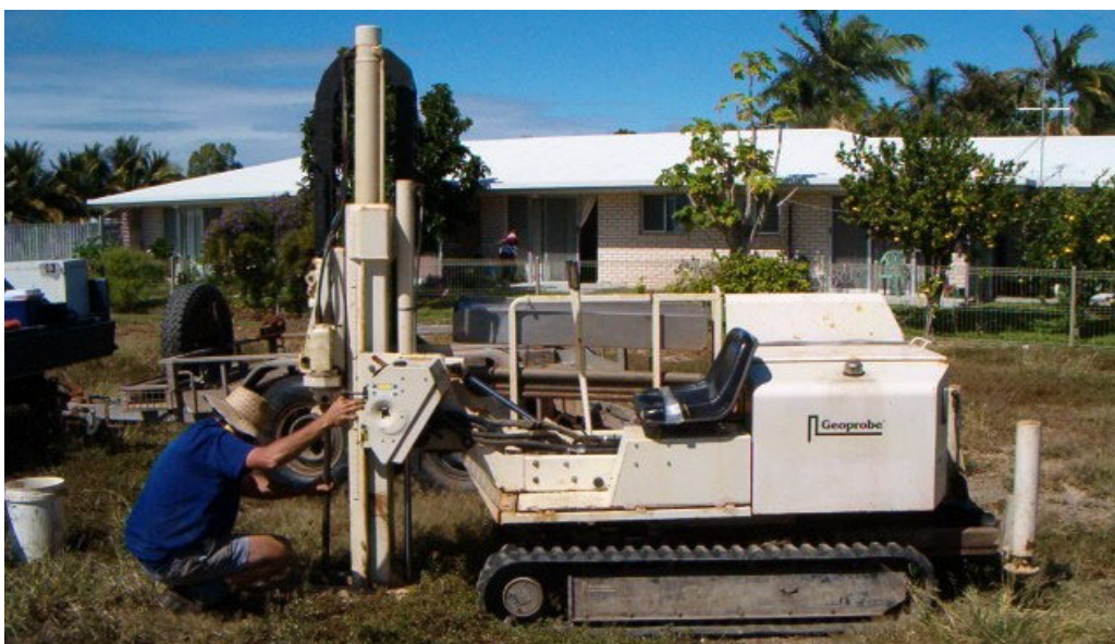
Photograph 4. Geoprobe ® used for deep sediment sampling
