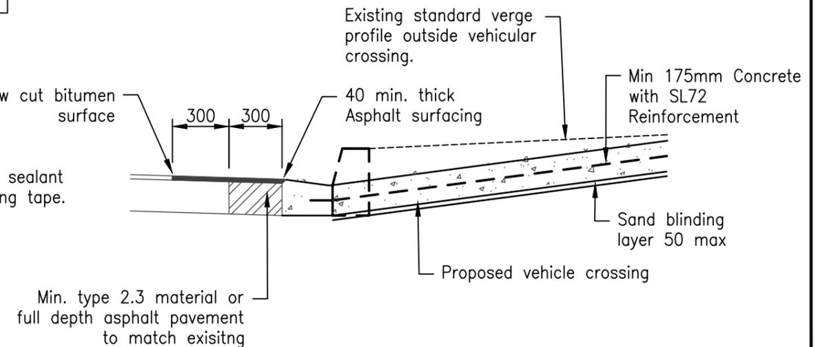
**TYPICAL SECTION - CHANNEL REMOVED**
