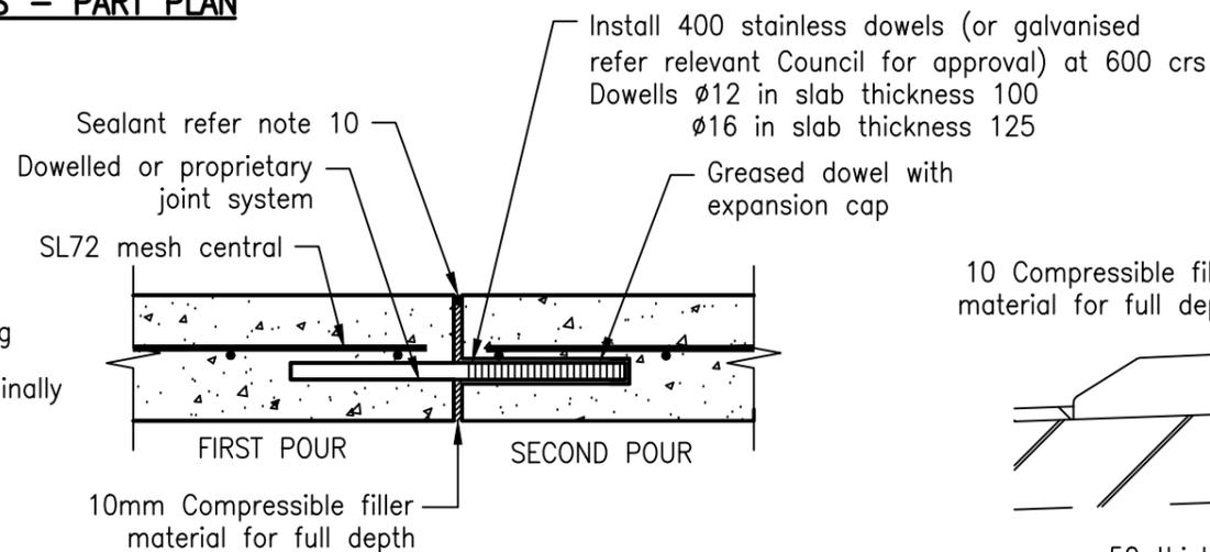
**DOWELLED EXPANSION JOINT DETAIL (DEJ)**
