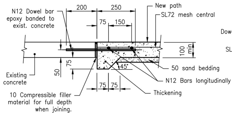
Dowel bars to be placed along the pathway midway between joints at 2000 crs, or as directed by the relevant Council
