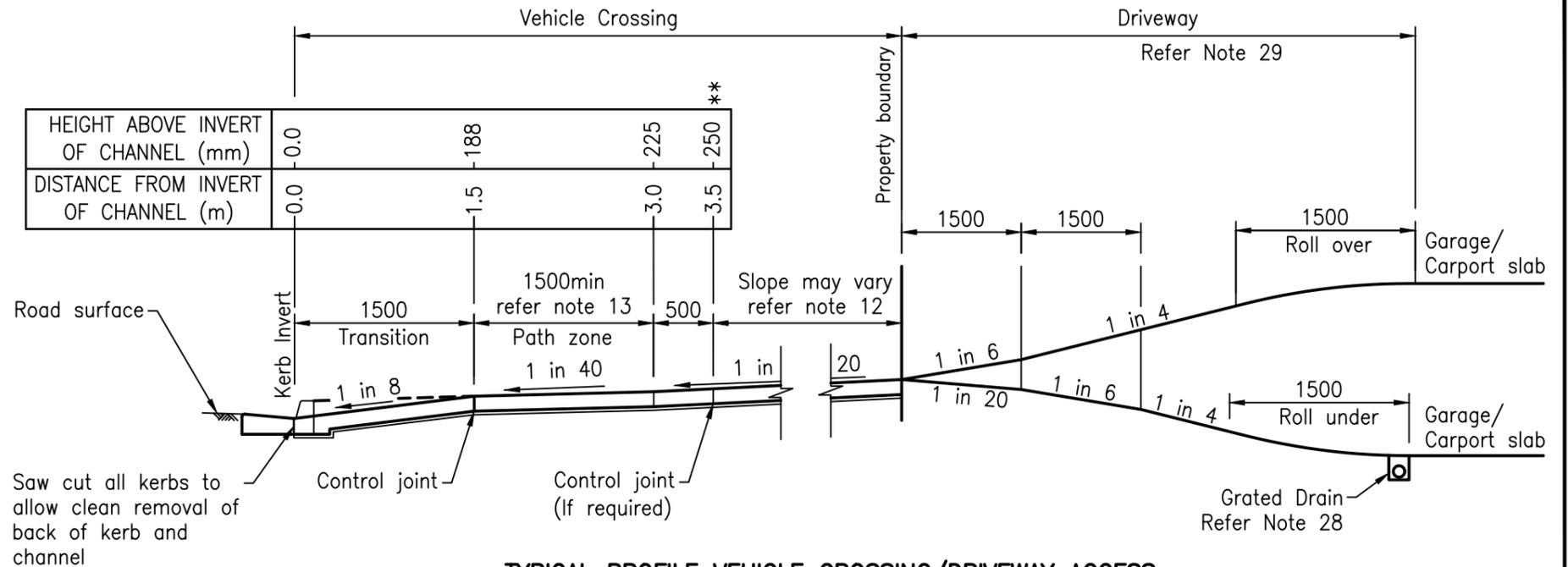
**TYPICAL PROFILE VEHICLE CROSSING/DRIVEWAY ACCESS SECTION B**
