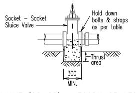
VALVE (SO-SO) - 300DIA OR LESS ELEVATION AT FITTINGS
