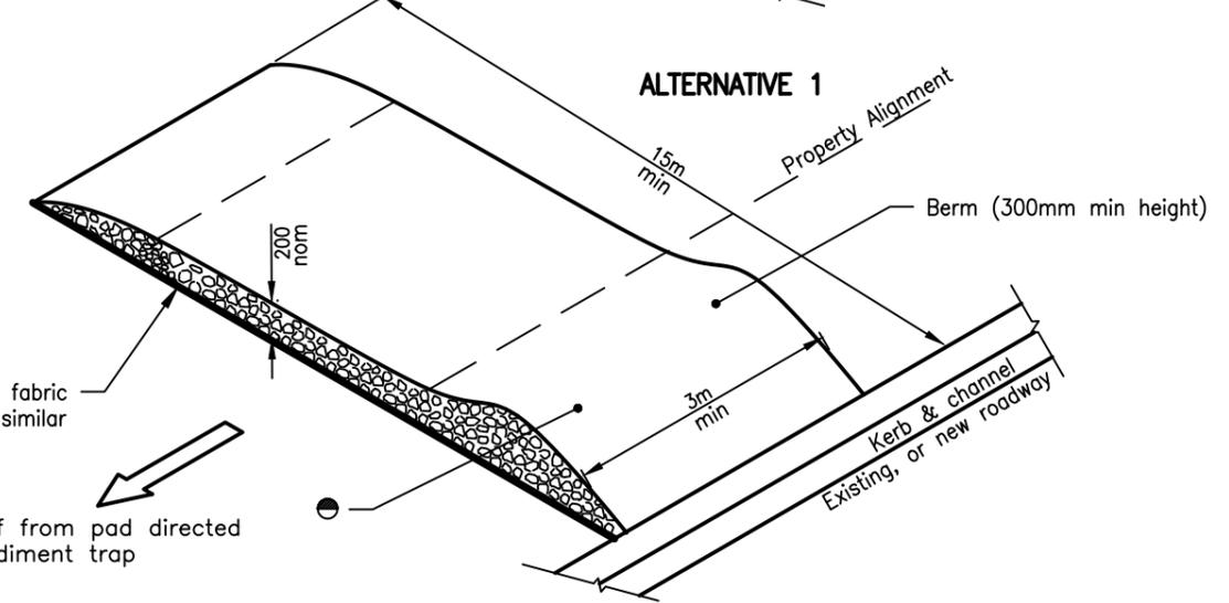
**TEMPORARY CONSTRUCTION ENTRY/EXIT SEDIMENT TRAP**
