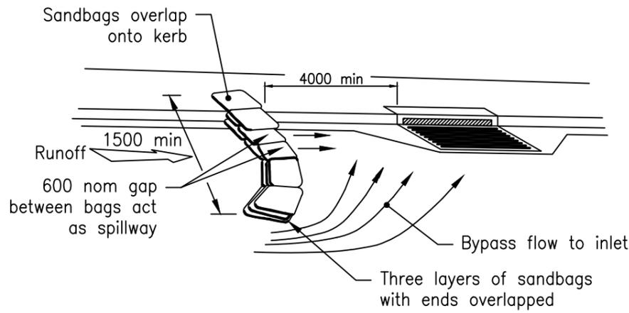
**ON GRADE KERB INLET SEDIMENT TRAP**
